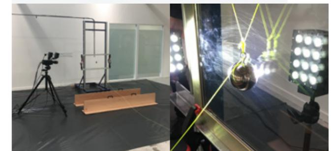
High speed camera test facility
